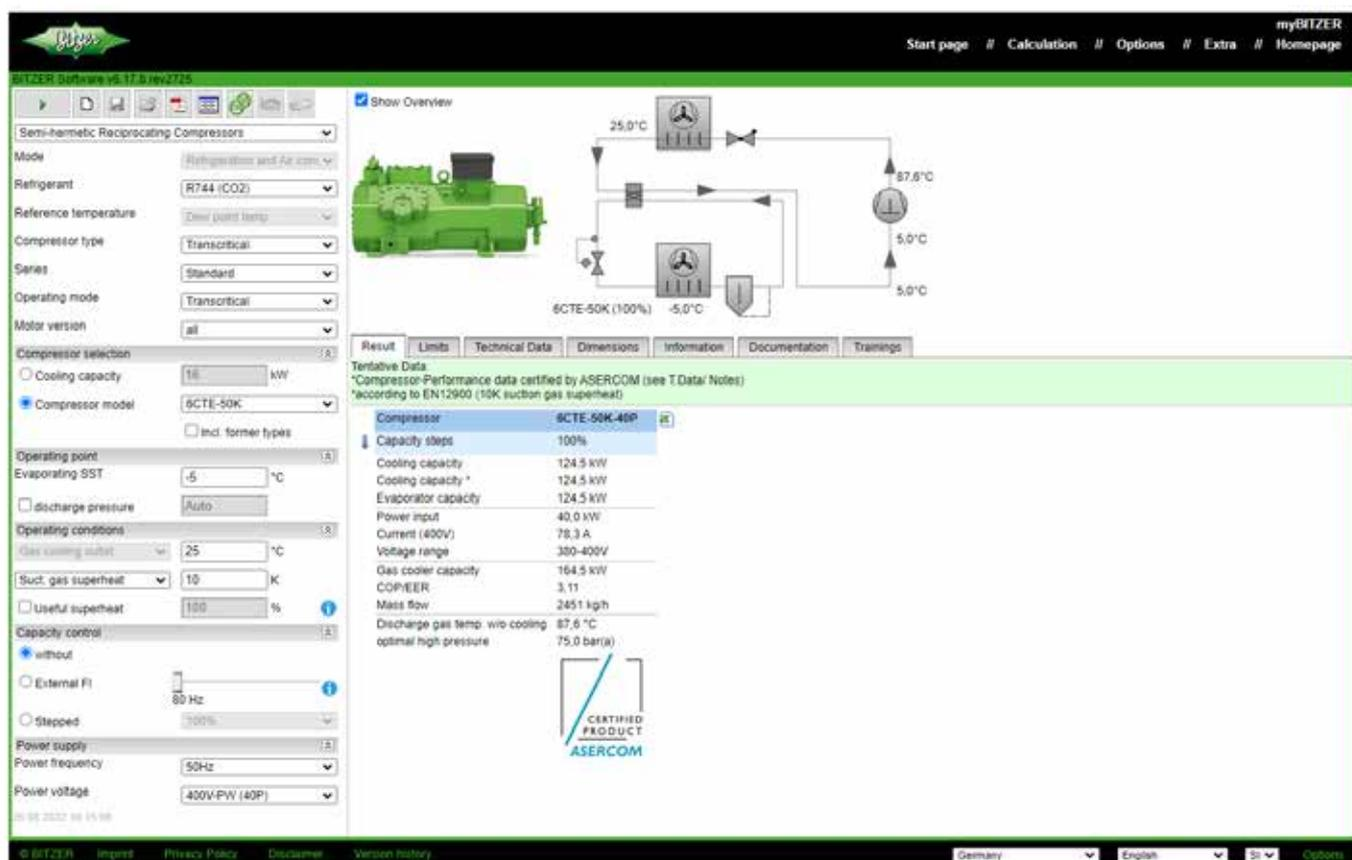
The screenshot displays the BITZER Software interface for selecting and calculating compressor performance. The left sidebar contains various configuration options, and the main area shows a schematic diagram of a refrigeration cycle and a table of technical data.
